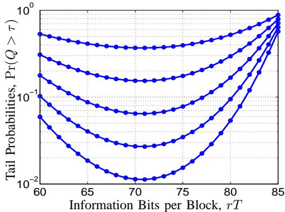
Fig. 3. This figure shows tail probabilities in the equilibrium packet distribution of the queue,  $\Pr(Q > \tau)$ , for threshold values  $\tau \in \{5, 10, 15, 20, 25\}$ . These probabilities are plotted as a function of the number of information bits per codeword,  $rT$ . The minimum on each curves represents an optimal operating point, and they are achieved uniformly at  $rT = 71$ .
