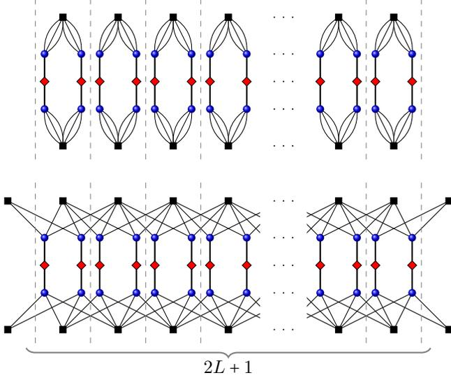
Fig. 5. Protograph of the joint decoder. Shown above are  $2L + 1$  copies of the protograph of the joint decoder for a  $(3,6)$  regular LDPC code. The bottom graph shows the protograph of the joint decoder for the corresponding spatially coupled code.
